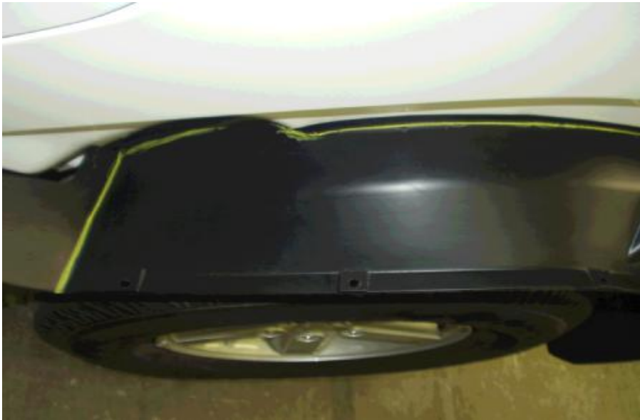
Figure #1- This photo shows the driver's rear fender liner marked for trimming. The view is of the front part of the liner.
