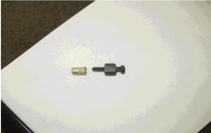
Fig. #4- Showing the rivet and the Expendable Tool
