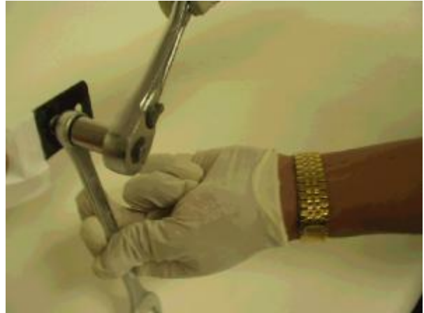
Fig. #5- Shows the tools needed to install the 1/4-20 rivet nut
